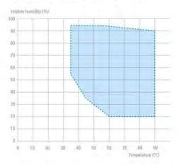
Note: Within the respective temperature-humidity range, permanent operation is possible (at an ambient temperature of 22 °C  $\pm$  3 K; relative humidity < 50 %). Condensation may occur in the threshold range. To which extent depends on the humidity content of the chamber load and the ambient conditions.
