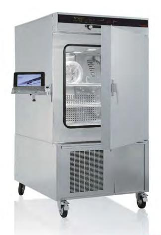
Climatic test chamber CTC with humidity control Temperature test chamber TTC "Celsius" standard software
