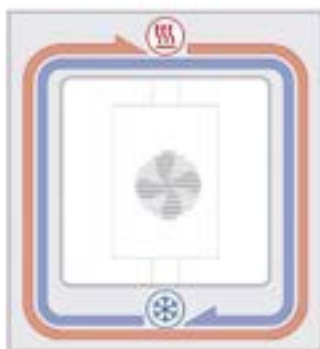
ICP air jacket temperature control system
